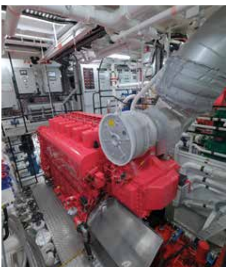
The main YANMAR 6EY26W engine.
