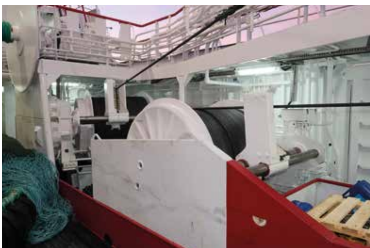
Starboard split winches.
