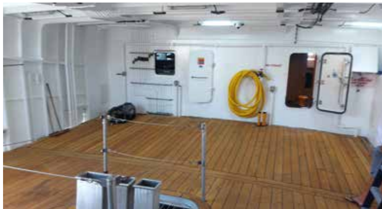
The cavernous under shelter deck area with timber sheathed deck
